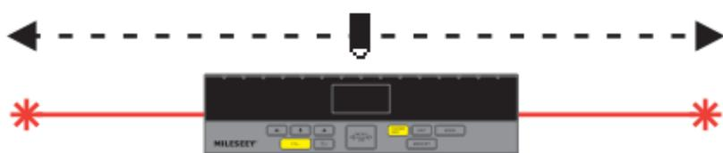
**Automatic switch to rear reference in case of one-way measurement.**
